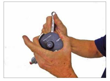
To Replace the disc, hold the disc firmly with one hand then turn the arbor with a wrench to loosen.
