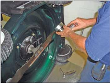
To grind, connect the grinder to an air supply. Position the guide on the bottom of the blade. Pull the trigger and pull the grinding disc across the blade while holding the guide against the bottom of the blade. Repeat as necessary.
