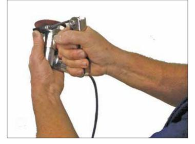
To set the grind angle, loosen the guide clamp with an allen wrench, set the angle of the guide and then retighten the guide clamp.
