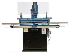
55001-01 The optional carriage drive is powered by a sealed, permanently lubricated rodless pneumatic cylinder with a self draining filter regulator. This makes the carriage drive virtually maintenance free. It can be purchased with the grinder or easily added at a later time.
