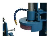
60690-10 The coolant mist system gives optimum cooling while using once through, always clean coolant.
