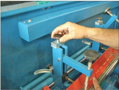
Tighten the bed knife clamp. Do not overtighten.
