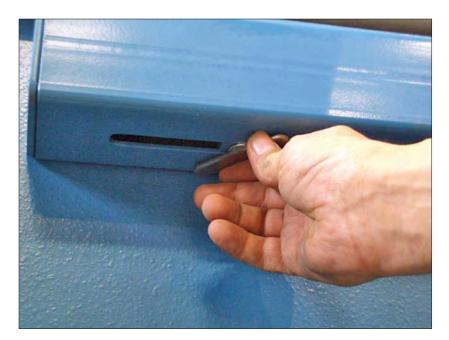
The travel stops are set by loosening the locking screw, positioning the stop and retighen the locking screw.
