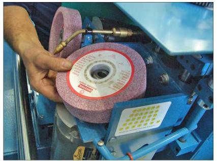
Place the new grinding wheel on the hub.
