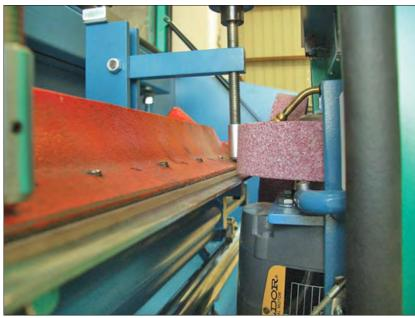
it just touches the bed knife. Move the grinding head across the bed knife. There should be even contact all the way across unless the bed knife is badly worn. If the contact is not even, recheck your set up. Repeat for the front face.
