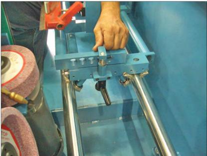
Rotate the clamps over the pallet.
