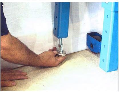
Mount the leveling pads provided in to the five legs of the grinder.
