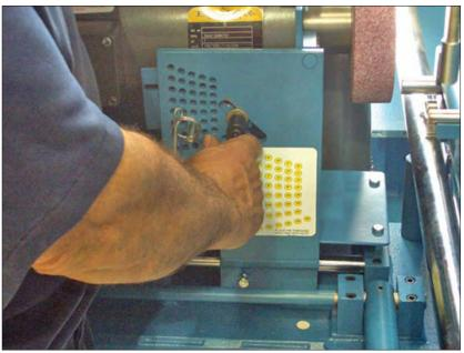
Unclamp the grinding head.
