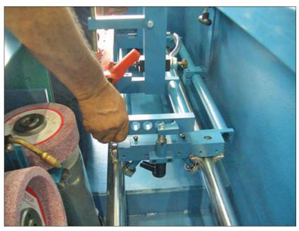
Lift up the right end of the pallet the set it back down. This ensures the left end is properly seated.
