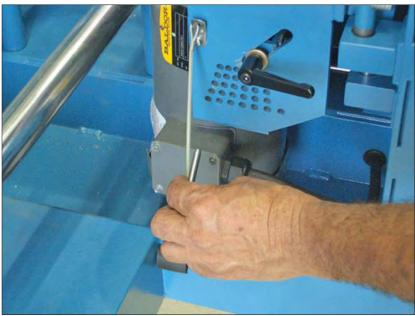
Remove the positioning pin.
