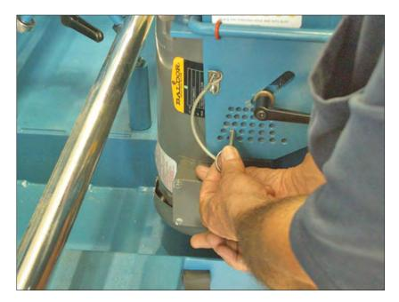
Using the chart, determine which hole will be used for the desired relief angle. Move the head so that the pin goes through the desired hole and into the slot attached to the motor.
