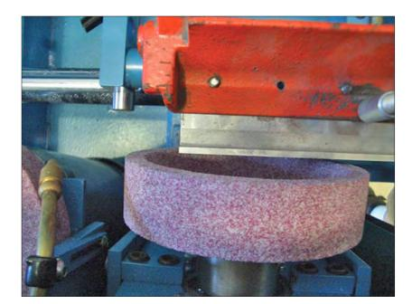
the part of the grinding wheels touching the bed knife (the inside edge) clears the ends of the bed knife.
