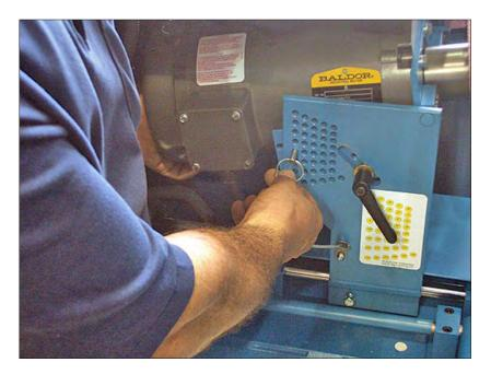
Using the chart, determine which hole will be used for the desired relief angle. Move the head so that the pin goes through the desired hole and into the slot attached to the motor.
