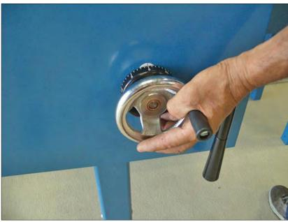
Adjust the hand wheel so the grinding stone is just touching the bed knife.
