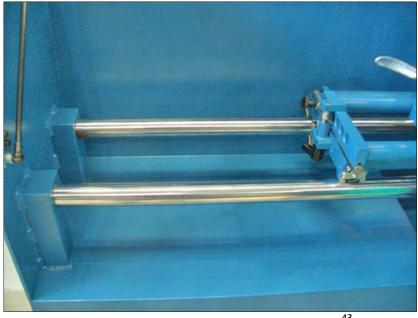
The track shafts must also be kept clean and free from grinding dust and are equipped with integral wipes. Do not oil the track shafts as that will cause the grinding dust to cling to the track shafts and make the wipes ineffective.
