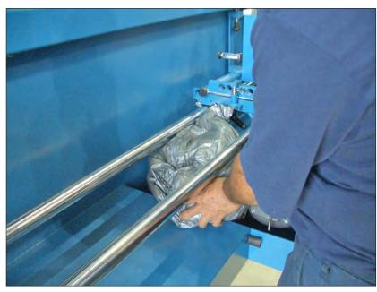
Remove all packing material from around the grinding head.
