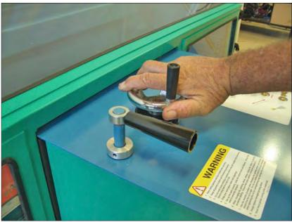
it starts to grind. Continue infeeding the grinding wheel until it is grinding all the way across the bed knife.
