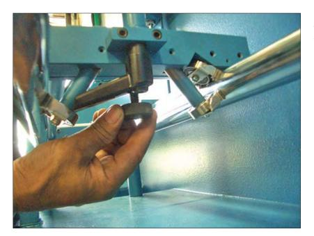
Infeed the vertical adjusting screw until the top is about even with the top of the vertical alignment pad.
