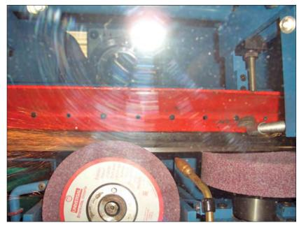
Continue infeeding left grinding head until the top face is done. Let the top face spark out after you have completed the front face.
