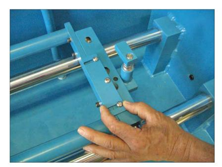
Slide the pad to expose the vertical adjusting screw.
