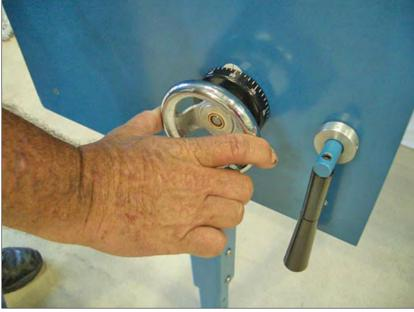
it starts to grind. Continue infeeding the grinding wheel until the front face is done.
