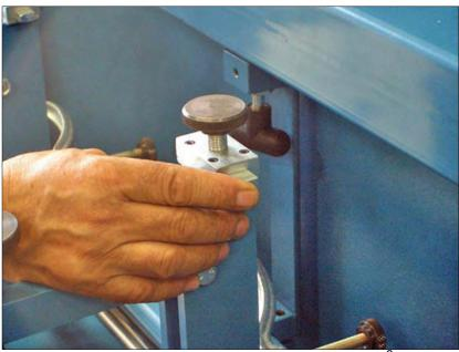
Push the button on the side to unlatch the arm.
