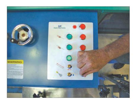
This controls the air flow for the coolant mist.
