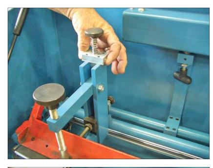
Swing the clamp arms up and remove the bed knife.
