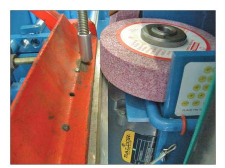
until the grinding stone is over the bed knife surface to be ground.
