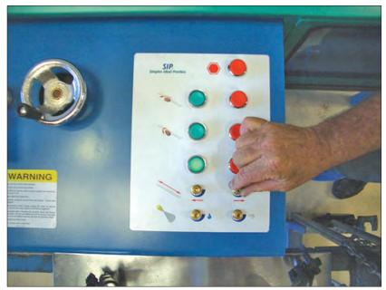
This controls the carriage speed. This is a needle valve which lets air bleed from the cylinder. Opening the valve counter clockwise increases the speed. Closing the valve clockwise decreases the speed.
