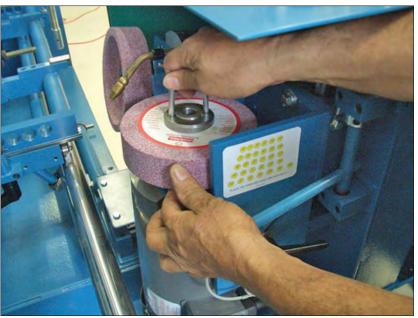
Tighten with the u-wrench provided. Do not overtighten as you may damage the grinding wheel. Use extra caution when turning the grinding motor on and off the first few times after you have mounted the grinding wheel. If the nut is not tight enough, it and the grinding wheel may come off when you turn the motor off.
