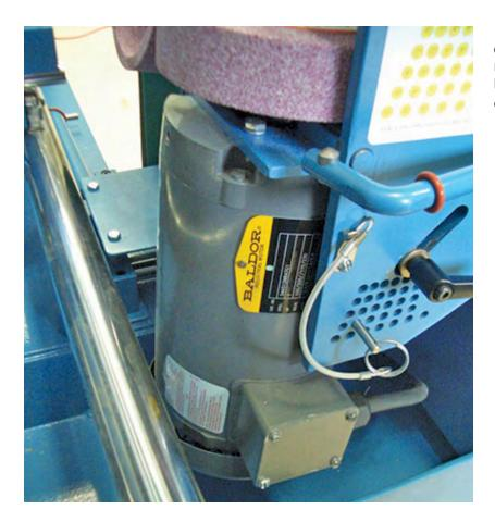
The grinder is equipped with totally enclosed fan cooled motors which require no regular maintenance. The motors should be cleaned periodically with either a vacuum or compressed air.
