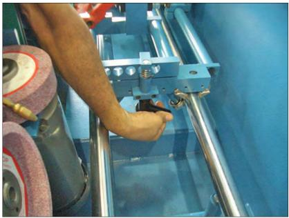
Unlock the backstop screw. Position the backstop against the pallet then tighten the screw.
