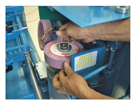
Using the u-wrench provided, hold the grinding wheel and unscrew the wheel nut. The left grinder is counterclockwise to loosen. The right grinder is clockwise to loosen.
