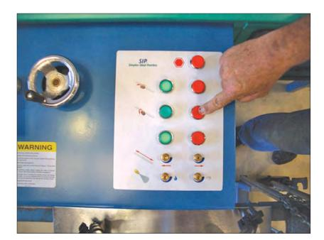
Back off the front face right grinding wheel and turn the right grinding motor off.
