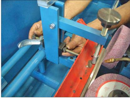
While turning the grinding wheel, adjust the back support screw until you have the same contact on both ends.
