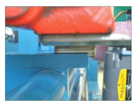
Make sure that the rear flat of the bed knife is resting on the shaft and...
