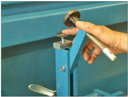
Place the bed knife on the supports, then unclamp the rear support. Position the rear support to a suitable height on the back of the bed knife and reclamp.
