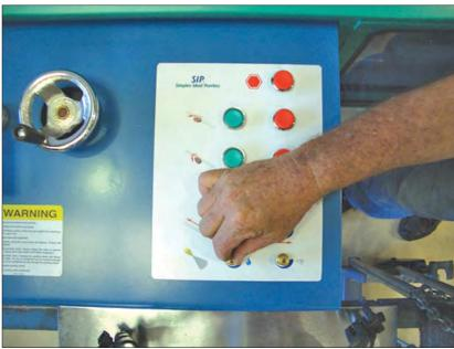
This controls the liquid flow for the coolant mist. The coolant mist comes on when the carriage travel is turned on. If you want to operate one without the other, close the valves of either the carriage travel or coolant mist to turn it off.
