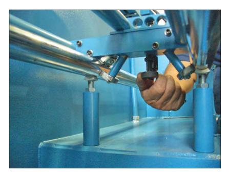
Adjust the vertical adjusting screw until the bed knife has equal contact on both ends.
