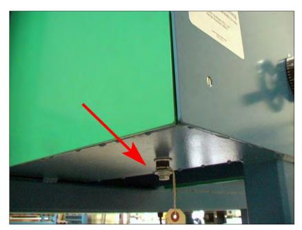
Remove the bolt which holds the counterweight for transport.
