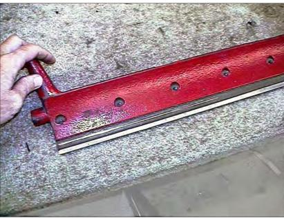
Inspect for a wavy appearance or condition along the top face of the bed knife. This would indicate that the bed knife has been adjusted to the reel with excessive pressure. This could cause worn or loose reel bearings.
