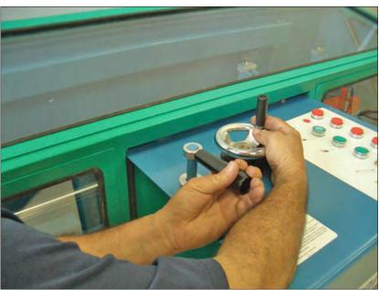
Turn on the top face motor, then infeed the grinding head and swing the dresser until no sparks appear. Turn off the top face motor
