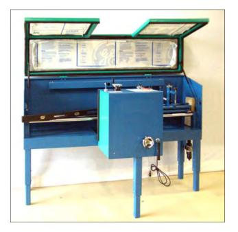
Lower the grinder in its final location. Check the grinder for level using a good quality carpenters level.
