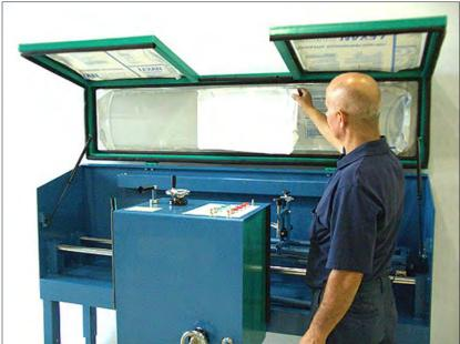
Remove the protective film from the Lexan panels
