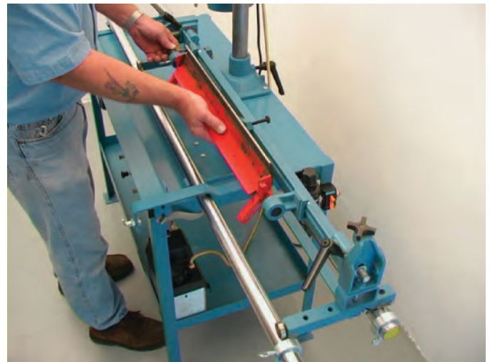
Place the bed knife between centers, aligning the mounting holes with the centers.
