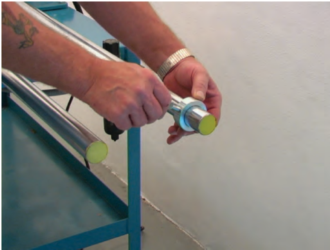
Mount the carriage stops on the track shafts.
