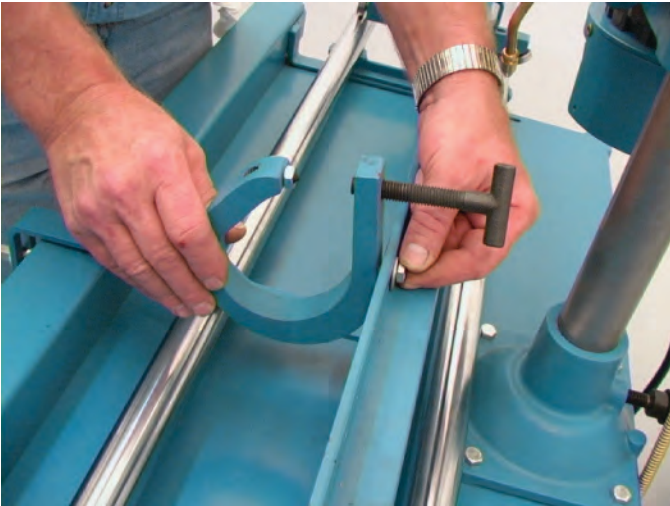
Mount the first clamp using the bolt and washer.
