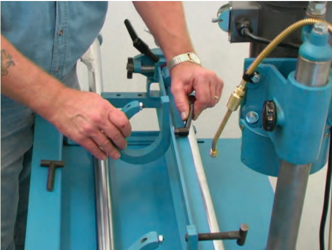
Mount the second clamp using the locking handle.
