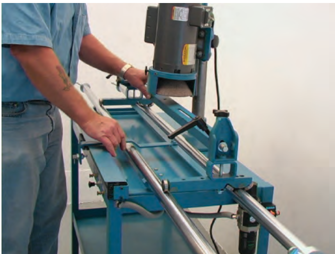
Place the carriage on the track shafts.
