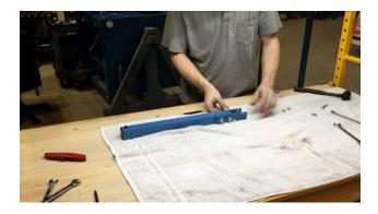
14. Attach the shelf brackets using the 3/8-16 x 2-1/2 bolts, nuts, washers and lock washers so that the hole closest to the shelf is on the bottom. Put a third bolt in that hole. Leave nuts finger tight.
