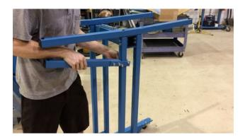
15. Place each shelf on a column and insert the final bolt with a washer, lock washer and nut.
