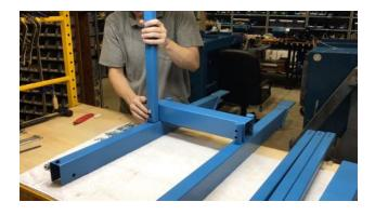
7. Place a column over a post and align the holes. Fasten using the 3/8-16 x 2 hex head bolts, lock washers and nuts. Tighten the nuts finger tight. Repeat for the other three columns.
