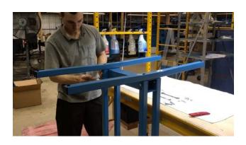
11. Position the top cross member (the one with the label) between the columns, align the holes using the  $3-8/16 \times 2$  hex head bolts.
