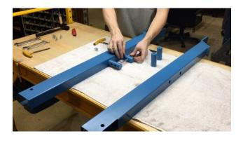
3. Align the holes of both posts using the long 3/8 bolt then tighten the bolts. Remove the long bolt.
