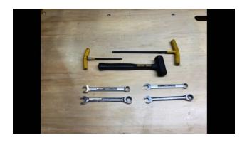
1. Tools needed: 2 - 9/16 wrenches, 2 - 1/2 wrenches, 1 - 1/4 allen wrench, 1 - 5/16 allen wrench, 1 - hammer. Watch the video at http://www.sipgrinder.com/videos/rackassembly.html
