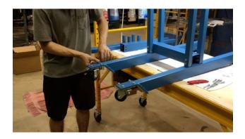
9. Mount the casters to one end of the leg using the  $5/16-18 \times 1$  hex head bolts, washers, lock washers and nuts. Tighten the bolts. Place the rack on the floor to complete.
