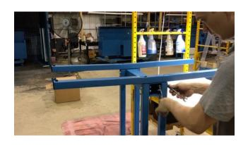
12. With all four wheels touching the floor, tighten the bolts on both the top and bottom of the columns.
