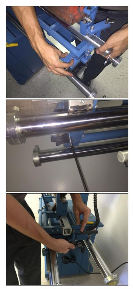
Slide or remove the pad to expose the vertical adjusting screw. Retighten the two screws.
