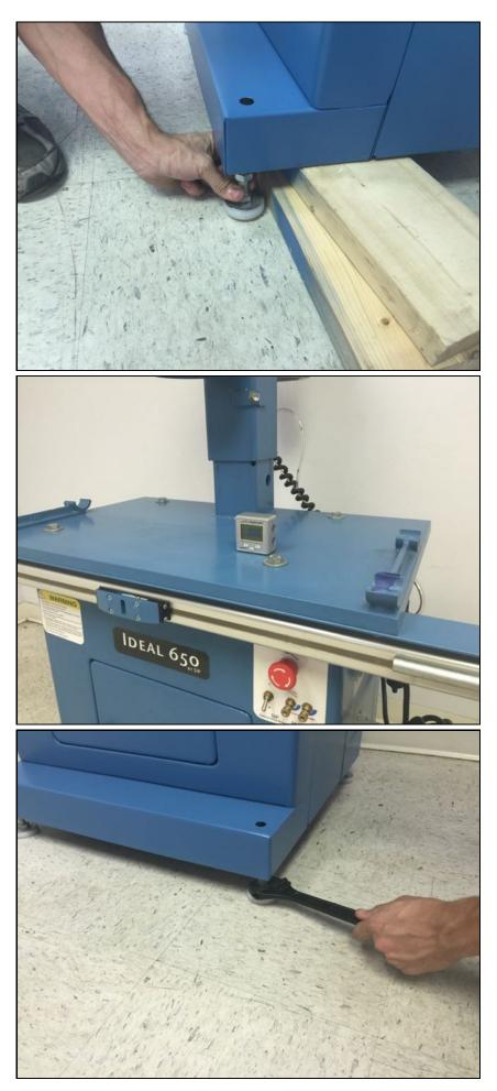
**2.2 Assembling the Grinder** Mount the leveling pads provided in to the four corners of the grinder.
