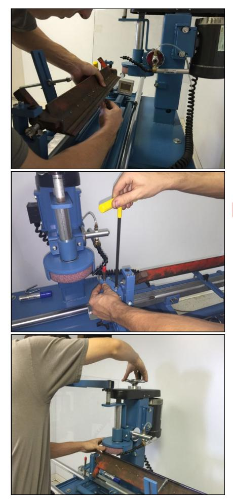
If the scratch is heavy on the front of either a new or used blade, then you may need to adjust the angle to compensate or dress the grinding wheel.
