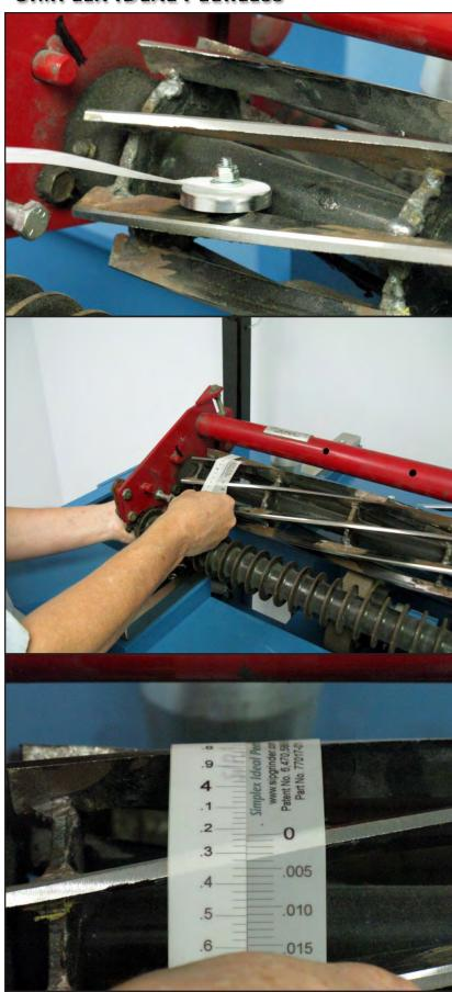
Place the magnet of the pi tape on a blade reel.
