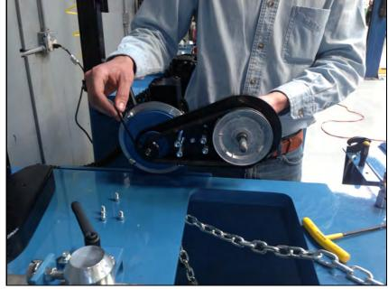
半径腕に設定ネジを緩めてください Loosen set screw in the end of the radius arm.
