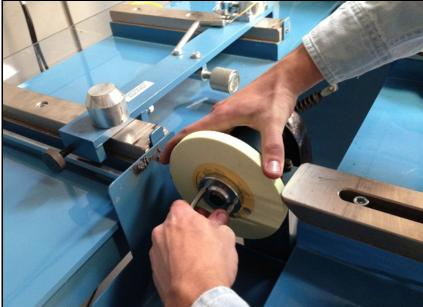
6.6 Aligning the fence Disengage the grinding head.
