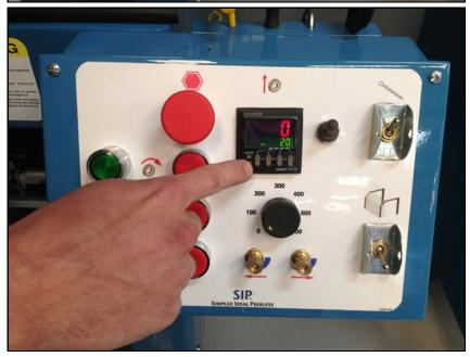
Turn the grinding motor on.
