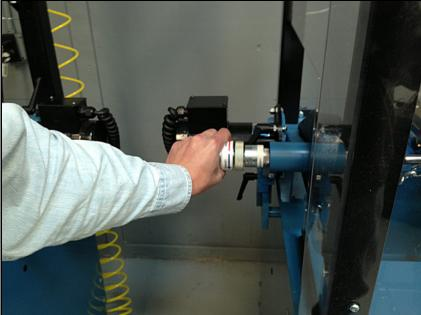
Rotate the slip clutch so you pull the blade away from the blade stop. Let go and make sure it pulls the blade back on to the blade stop.
