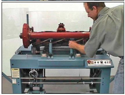
Adjust the support stands as necessary. Then retighten the frame or roller mount.
