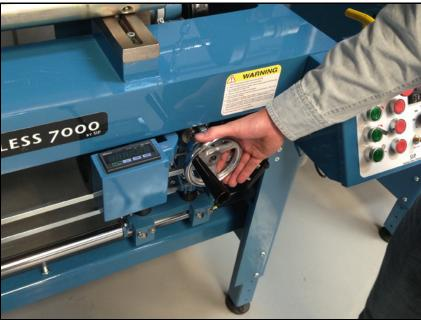
Move the grinding head to the right end of the reel...
