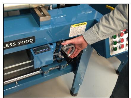
Move the grinding head to the right so that both the blade stop and the indexing stop are against the reel blade.
