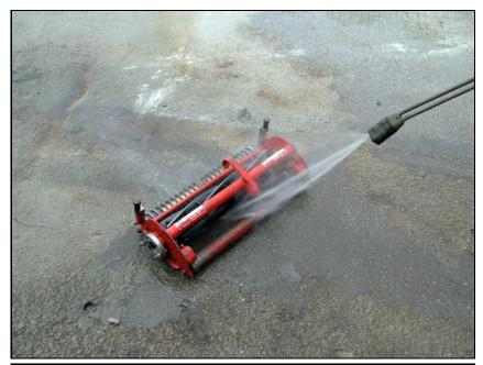
3.0 Prepare the cutting unit for grinding Clean all dirt, grass, rust, grease, and oil from the mower assembly, especially where it accumulates behind the lip of the bed knife.
