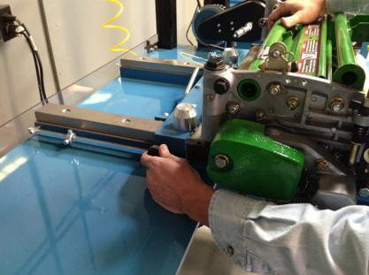
Bring the rear fence up to the rear roller. Lock down the left side making sure that the fence aligns itself.
