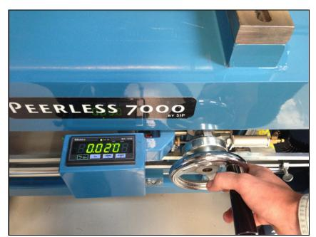
While turning the lawn mower blades, adjust the front roller until the grinding stone just touches the reel.
