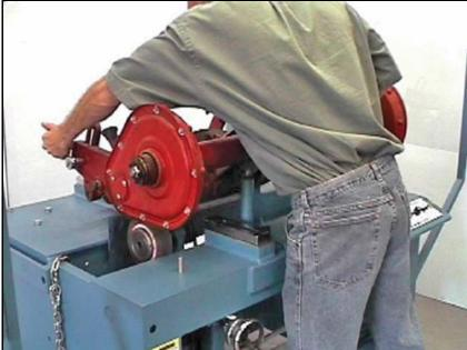
Use the optional support stands for cutting units without a front roller. To adjust the cutting unit, loosen the frame or roller mount.
