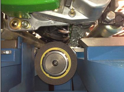
If it does not, loosen the two socket head bolts in the front reel support rail and slide the rail back. Retighten the socket head bolts.
