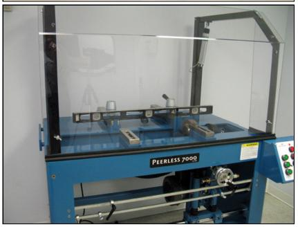
With the grinder in its final location, use a good quality carpenters level to adjust the leveling pads until grinder is level.
