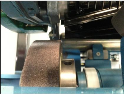
Move the grinding head to one end of the reel so that the grinding stone is just off the end of the reel blade and does not touch the cutting unit frame. If you can not clear the frame, you may leave all or part of the grinding stone on the reel.
