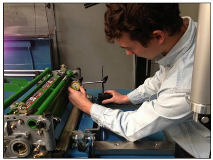
If you would like to be more precise, you can use the dial indicator and magnetic base. Slide the magnetic base front to back and find the high point on one end of the roller.
