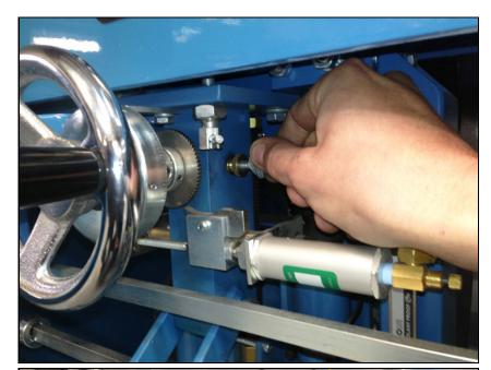
Snug the tension screw. Depending on the size, type, and condition of the reel, you may wish to adjust the speed of the spin motor or the carriage travel so that you get a smooth, consistent grind.
