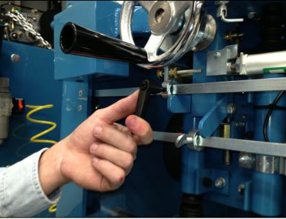
With the left lever in the up position, set the top left carriage travel stop.
