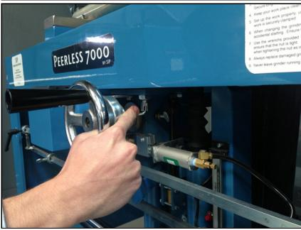
6.1 Aligning the head vertically
