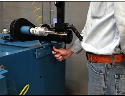
Clamp it in place. The clamping knobs are ratchet style handles and can be adjusted by pulling out and turning.
