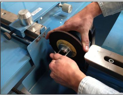
For the relief grinding stone, use the u-wrench provided, hold the stone and unscrew the wheel nut counterclockwise.
