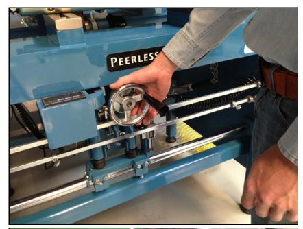
Move the carriage past the reel support rails and make sure there is adequate clearance between the grinding stone and the reel support rail.
