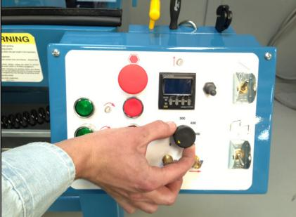
Turn the reel drive motor on.
