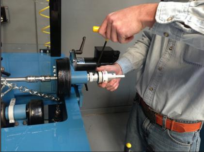
Align the clutch set screw with the clutch lock-out set screw and tighten the clutch lock-out (inner) set screw on to the flat of the shaft.
