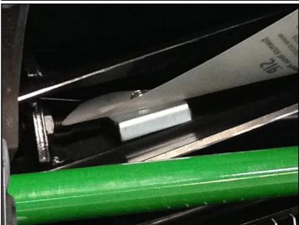
Make sure that the magnet is in far enough so that it will not touch the Reel Diameter Tape™ when you wrap it around.
