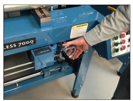
Move the grinding head back and forth across the reel and check for correct function of the blade stop and indexer.
