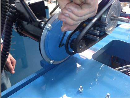
Rotate the arm around the eccentric to loosen or tighten the belt.
