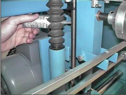
The feed screw should be lubricated lightly with dry graphite as needed for easy operation.
