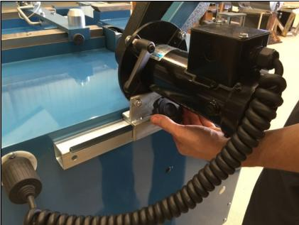
Hold the reel drive motor with one hand and loosen the locking knob which clamps the unit to its support.
