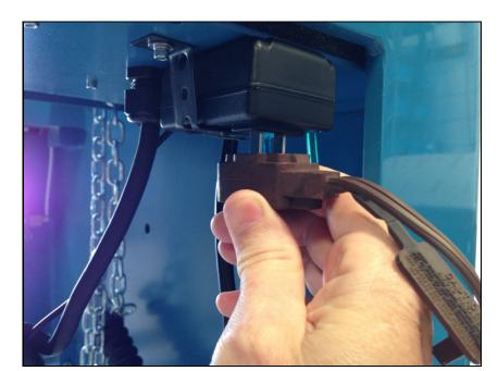
If you have the optional Digital Readout, plug an extension cord to the transformer plug on the bottom of the back panel.
