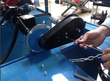
6.8 Adjusting the grinding motor belt Loosen bolts which mount the motor. Slide the motor up or down. Re-tighten the motor bolts.
