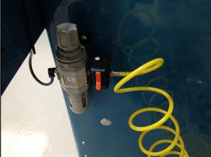
2.4 Connecting the service Connect the air supply to the filter regulator Set the pressure to 70 psi.
