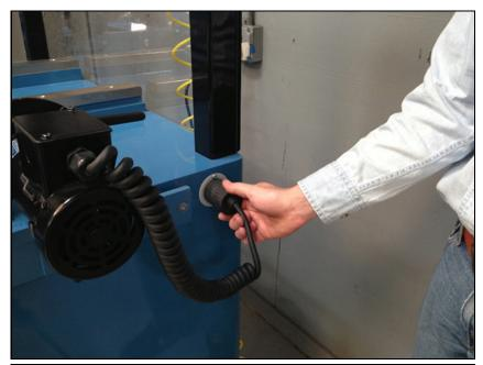
Plug and twist the motor plug into its receptacle on the same side as the reel drive motor is mounted. The reel drive motor is smart wired so that it will always rotate in the correct direction. The cord is only long enough to plug the motor into the side on which the reel drive motor is mounted. mounted.
