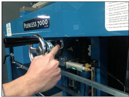
4.0 Setting the carriage stops for spin Disengage the grinding head from the carriage travel by pulling then turning the locking pin.
