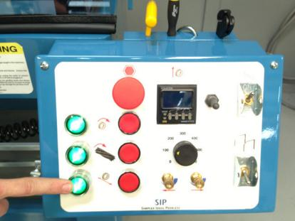
You may need to adjust the speed to get a satisfactory grind. Most of the grinding is done as the grinding stone feeds into the blade. This will be as the grinding head is moving to the right for right hand spiral blades and to the left for left hand spiral blades.
