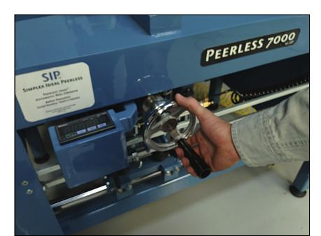
Move the grinding head to the left end of the grinder.
