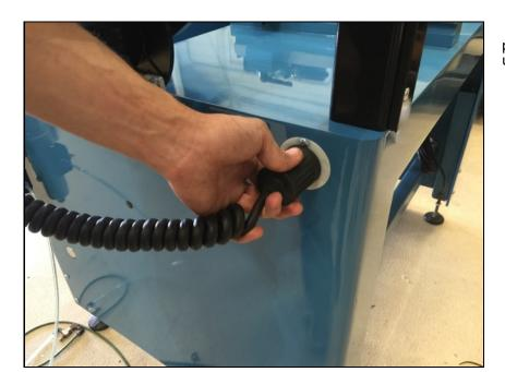
Plug and twist the reel drive motor plug in its receptacle on the same side as unit is mounted.
