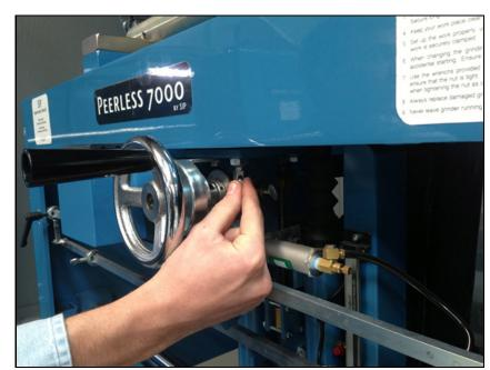
Engage the grinding head to the pneumatic drive.
