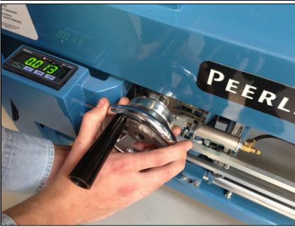
While holding the hand wheel, turn the dial until it reads 0.
