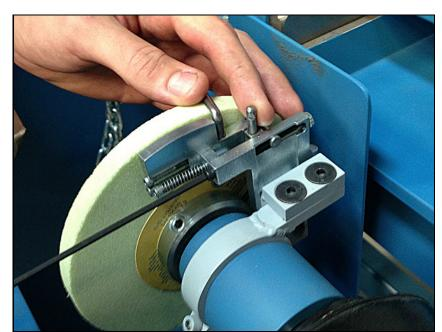
To set the indexer forward stop so that it is caught by the blade during indexing, adjust the screw on the right.
