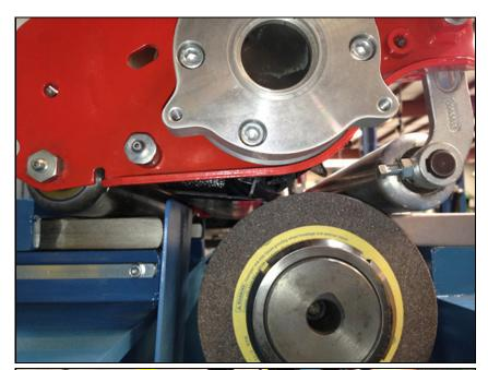
If you are grinding with the bed knife in place, locate the reel so that the grinding stone will only grind the reel blades and clears the bed knife, front roller, and any other part of the reel.
