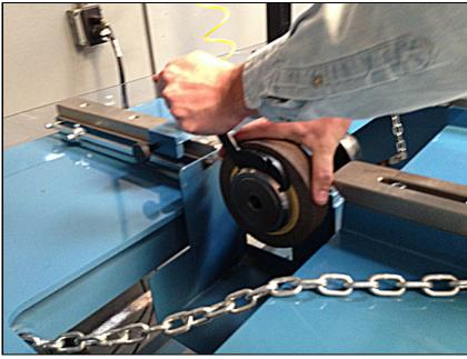
For the spin grinding stone, use the spanner wrench provided, hold the stone and unscrew the wheel nut counterclockwise. Remove the stone.
