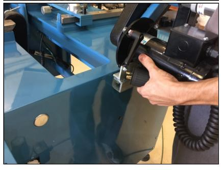
Lift the assembly off the support, turn it around, and place it on the support at the other end of the grinder.
