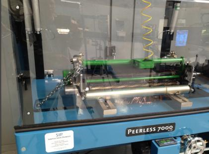
The auto infeed will continue to feed the grinding stone. Listen for uniform grinding sound all the way across the reel. When the counter has reached the total count you selected, it will stop infeeding and spark out. If the reel is not sharp you may reset the counter for additional passes. You also have full manual control of the grinding stone infeed, even in full auto mode.
