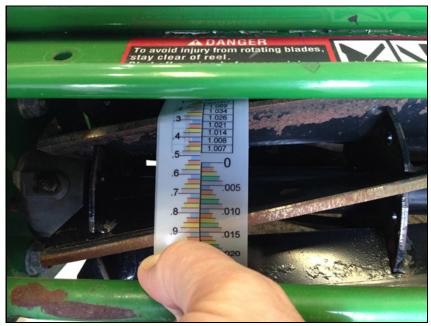
Make sure that you wrap it in a straight line so that the end of the tape lines up with the vernier line of the tape. Note the reel diameter, in this case, 4.534 inches.
