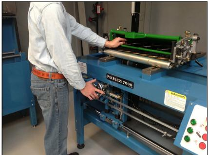
Feed the grinding stone up at the large end of the cutting unit while turning the reel until the wheel just touches the reel. You should do this at the same place you took your Reel Diameter Tape™ measurement.
