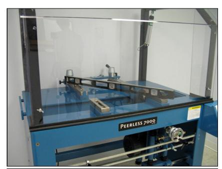
Again using the level, adjust the foot pads so that the back of the grinder is slightly lower than the front. This will let the reel roll into the fence.
