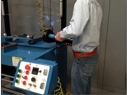
2.3 Reel drive motor Mount the reel drive motor.
