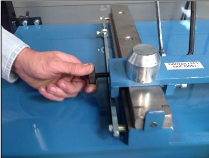
Lock the fence in position with the left side locking knob only.
