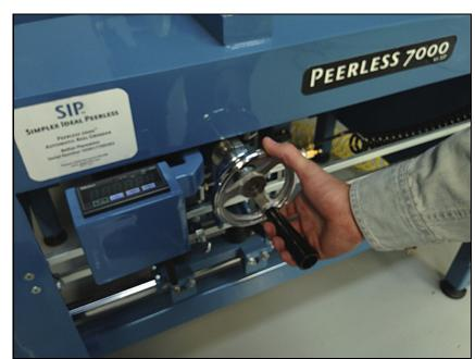
Check that it just touches by holding the reel blade against the blade stop and turning the grinding stone.
