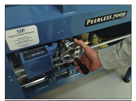
Adjust the grinding stone down 1 to 2 revolutions of the hand wheel for smaller reels and 4 or more revolutions for larger reels. Make sure that the relief angle does not exceed 45°. This will give approximate the correct relief angle for most reels. You may need to adjust up or down depending on your reels.
