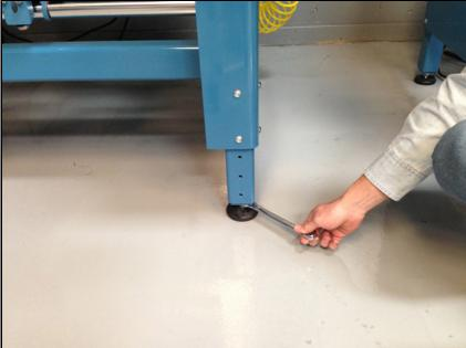
Mount the leveling pads provided in to the four corners of the grinder.
