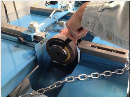
Replace the wheel nut and tighten with the spanner wrench provided. Do not over-tighten as you may damage the stone. You may remove the hub assembly and mount it carefully in a vise for tightening.
