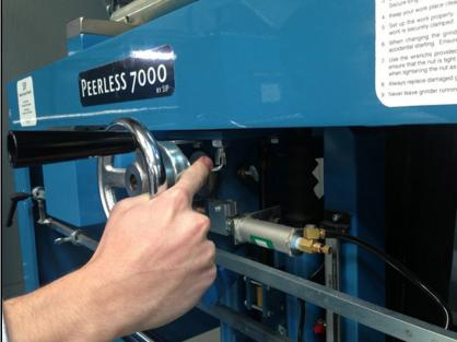
5.1 Remove the spin grinding stone Disengage the carriage travel.
