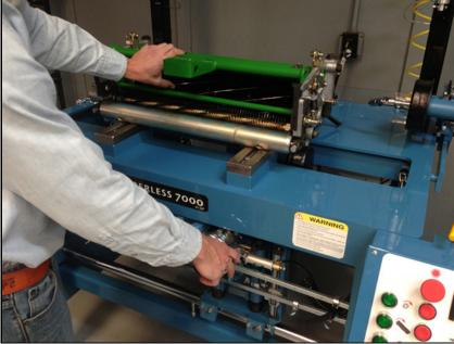
Infeed the hand wheel the difference in the left and right lawn mower diameters by reading .020 on the hand wheel dial...
