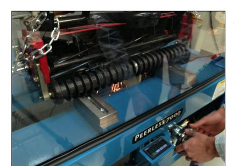
Feed the grinding stone up until it just starts to grind.
