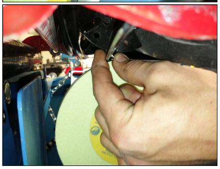
Squeeze the blade and blade stop together while pulling the blade against the grinding stone.
