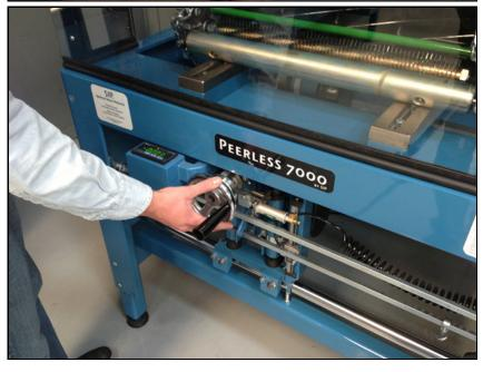
Slowly feed the grinding head in until the grinding stone starts to grind the reel then allow the grinding head to travel back and forth.
