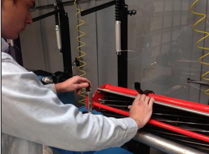
If the rear roller is fixed and the frame is bolted, first adjust the front roller as before.
