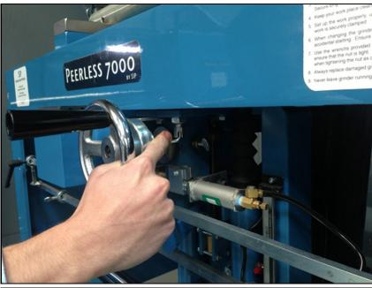
6.3 Dressing the grinding stone Disengage the grinding head. DANGER-Wear face shield! Stay clear of stone when starting machine!
