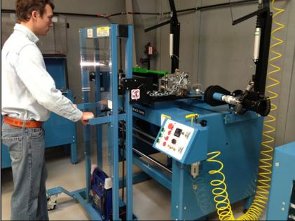
Place the cutting unit on the reel support rails.
