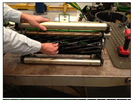
Check that the front spacer bar and that the bed knife is not loose. If the frame is loose, it is probably out of alignment. Check the mower manufacturer's manual to reset alignment.
