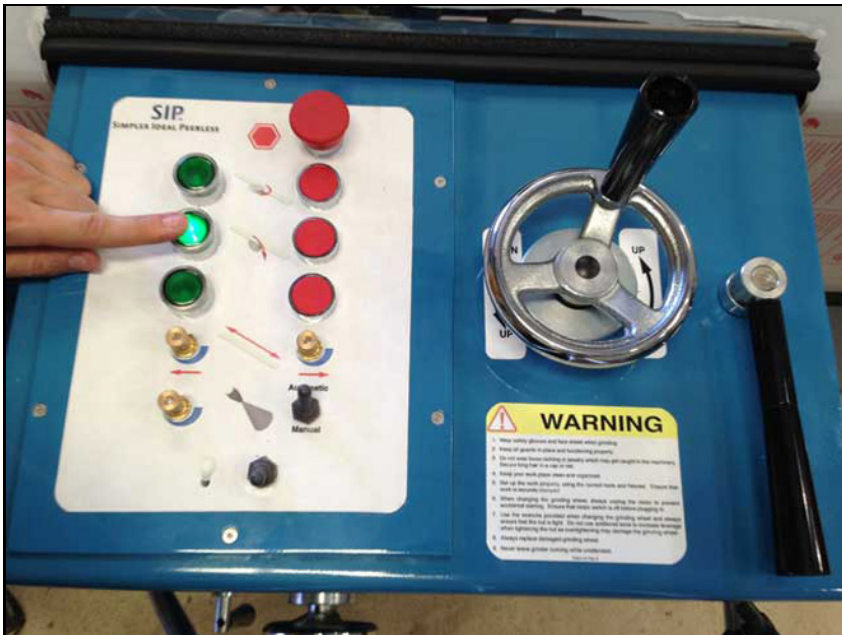
The front face grinding motor on and off buttons.
