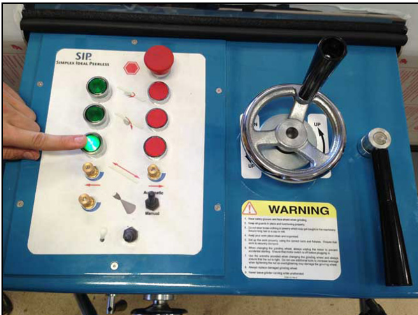
Carriage travel on-off. The carriage travel operates with air. This also turns the coolant mist on and off.
