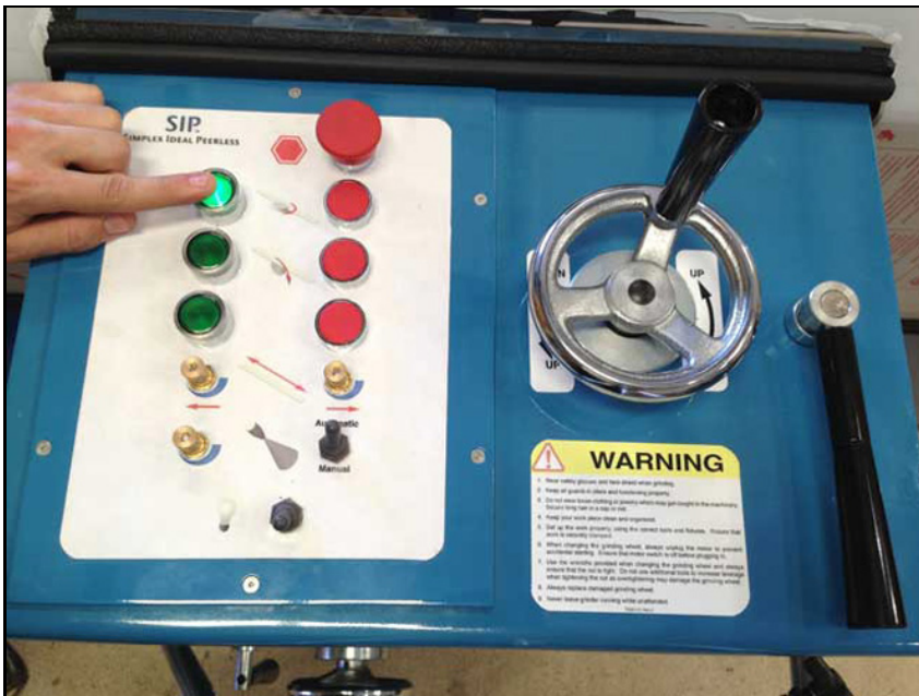
The top face grinding motor on and off buttons.
