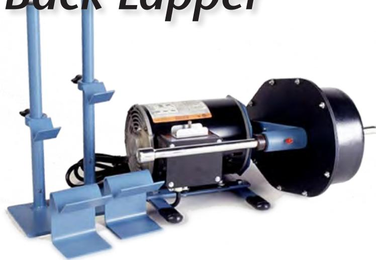
Thank you for selecting the Simplex 350 Lapping Machine. We believe it is the finest industrial grade lapping machine for reel mowers available. Made with heavy gauge steel and cast iron, glass filled nylon gears and a large 1/2 horsepower motor, the Simplex 350 will provide years of efficient, trouble free service.
