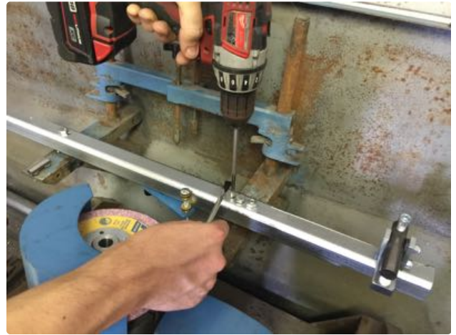
29. Ream the holes in the bar with the .249 reamer.
