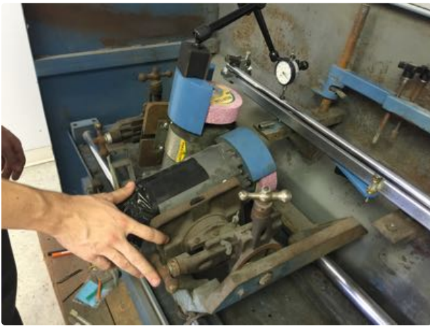
20. Reposition the dial indicator so that the tip of the indicator rests on top of the shaft.
