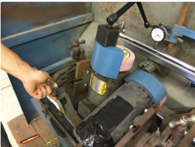
21. With the dial indicator over the main support on the left end, move the head in or out to find the high point of the shaft.
