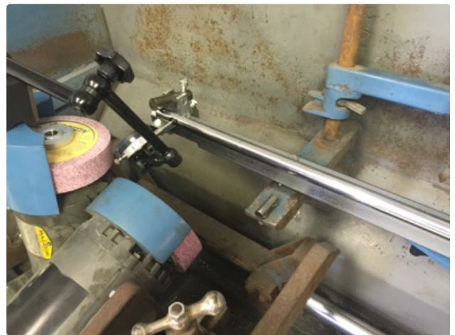
12. Place a dial indicator on a magnetic base on to a grinding head so that the tip of the indicator rests on the front of the shaft. Use a flat tip.
