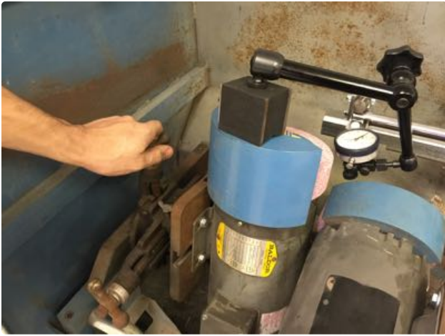
13. With the dial indicator just inside the v-support on one end, move the head up or down to find the high point of the shaft.
