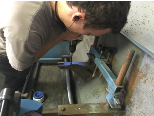
8. Remove the bar and drill the holes with a 5/16 drill at least 3/4 deep.
