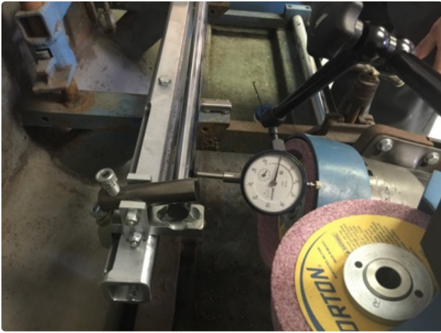
19. Move the grinding head back to the first end and repeat steps 13 through 17 until the difference is less than .003.
