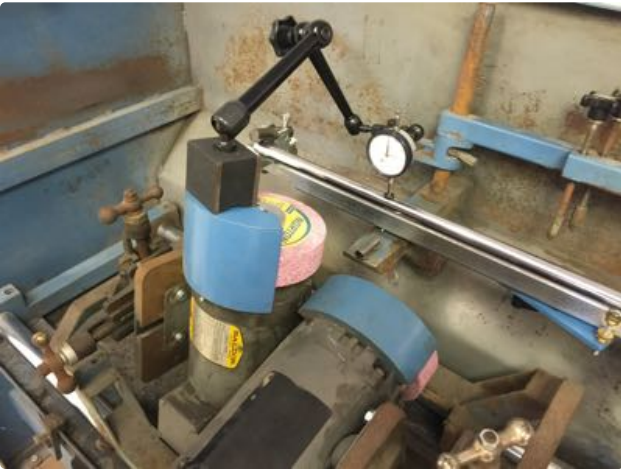
26. Move the grinding head back to the first end and repeat steps 22 through 25 until the difference is less than .003.
