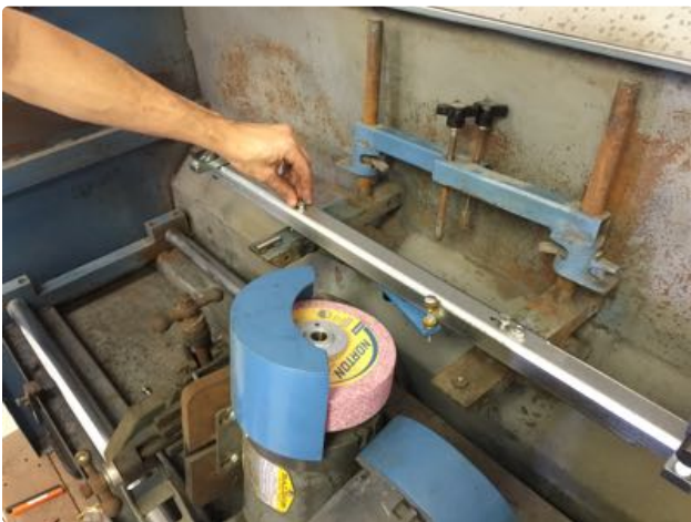
33. Remount the bar on to the bed knife support and double check its position.
