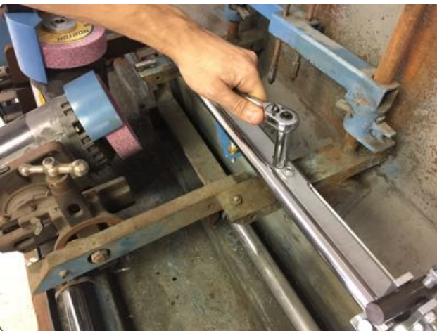
27. Tighten the bolts which hold the bar to the bed knife support, Then recheck both the top and front measurement to make sure they are within .003.
