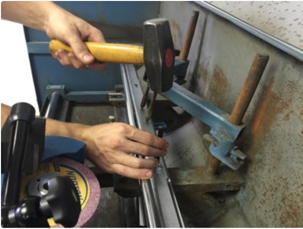
7. Transfer punch and center punch the hole location of the two large holes in the bar.
