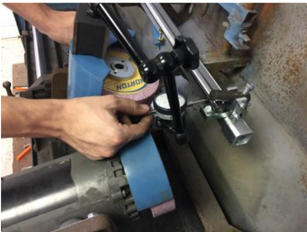
15. Pull back the dial indicator stem and move the grinding head to the other end of the roller shaft, just inside the v-support.
