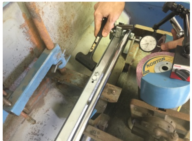
18. Tap the bar lightly on that end and move the bar half of the difference. If it reads .030, move the bar until it reads .015.
