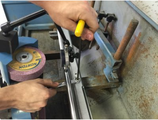
25. Loosen jam nut then adjust the bar up or down using the set screw until it is zero. Retighten jam nut.
