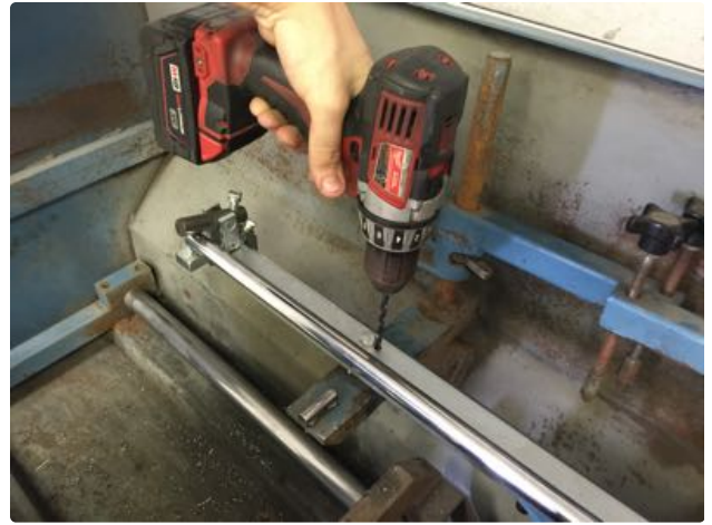
28. Drill through the dowel pin hole of the bar into the bed knife support with a 15/64 drill (provided in optional drill kit) at least 5/8 deep.
