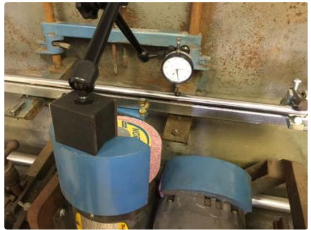
23. Pull back the dial indicator stem and move the grinding head to the right end of the roller shaft, just inside the v-support.
