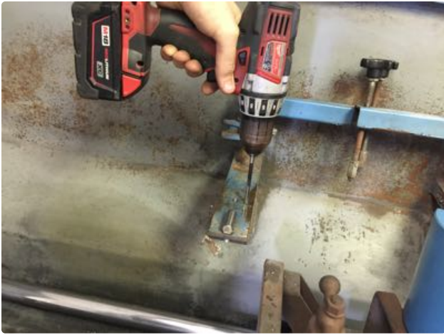
31. Ream the holes in the bed knife support with the .251 reamer.
