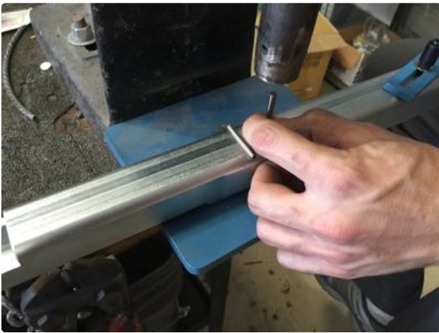
32. Press the dowel pins provided from the bottom of the bar into the .249 holes until they are flush with the top.
