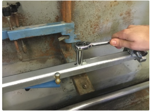
10. Replace the bar and bolt in place with the 3/8-16 x 2 bolts provided.
